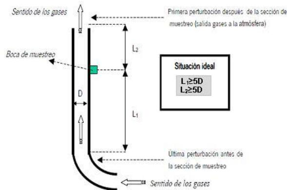
$$L_1 \geq 5D \text{ y } L_2 \geq 5D$$
